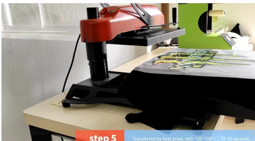
step 5 Transferred by heat press, with 120-150°C , 15-25 seconds
